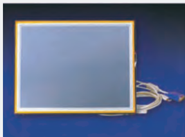
15" LCD TFT chassis. Resolution: 1024 x 768. Brightness 250 or 1500 cd/m 2 optional. Contrast 400:1. Analog input. Touchscreen optional.
