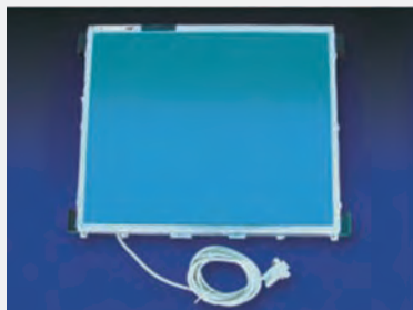
17" LCD TFT chassis. Resolution: 1280 x 1024. Brightness 250 or 1500 cd/m 2 optional. Contrast 450:1. Analog input. Touchscreen optional.
