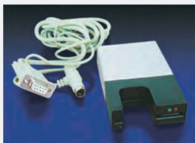
Manual Hybrid Card Reader SCR28. Smart, Memory and Magnetic Card Reader, Manual insertion Drivers and libraries for Windows, CE, Linux. RS232 or USB interface.
