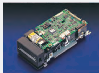
Motorised Hybrid Card Reader ICM330. Smart and Magnetic Card Reader, 1 SAM socket on board. Anti-Intrusion shutter. EMV Approval. RS232 or USB interface.
